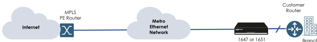
DIA (Direct Internet Access) service over L2
